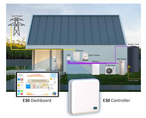
The tablet-sized E30 Energy Flow Dashboard<sup>™</sup> & Controller – links to household systems like switchboard, solar, battery, air-conditioning, drinking water, grid & smart appliances, for 'energy visibility', programming and AI decision-making.
